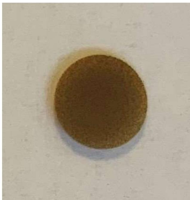
**Figure 2:** rGO-coatings on borosilicate glass-slide prepared by electrospaying.
