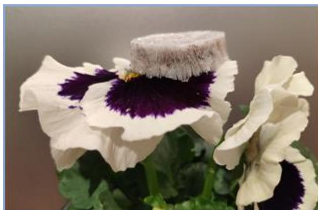
**Figure 1.** Image of a cellulose nanocrystal-based aerogel
