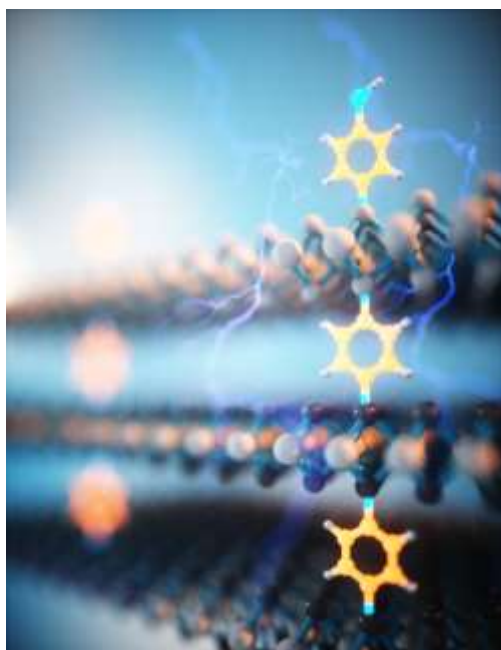
Figure 1: 1,4-benzenedithiol molecules simultaneously healing sulfur vacancies in solution-processed MoS_2 and covalently bridging adjacent flakes, to create percolation pathways for the charge transport in transistors.
